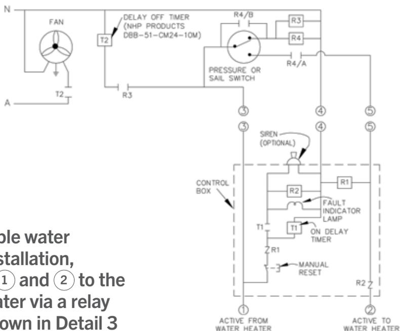
For multiple water heater installation, connect ① and ② to the water heater via a relay box as shown in Detail 3
