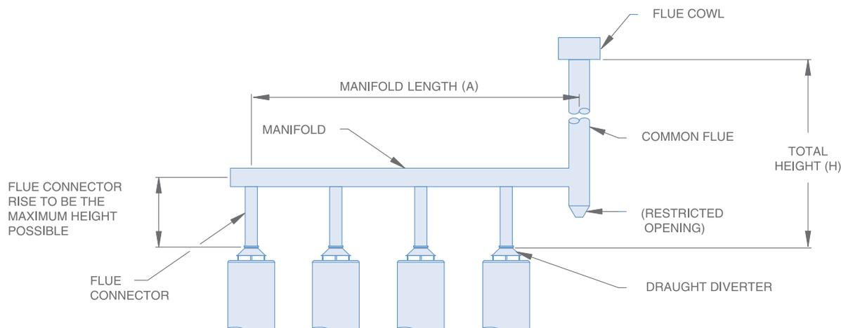
NOTES: The length of manifold "A" should not exceed 50% of total flue height "H".
