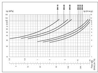
This chart shows curves at a 800kPa inlet pressure and 300kPa set pressure; curves for other settings are similar. The curve shifts slightly to the left for a smaller differential and to the right for a greater differential.
